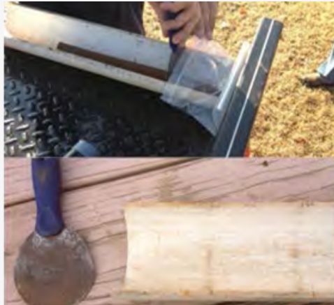
Figure 5: Rounded putty knife fits into the PVC cradle for cutting the core.
