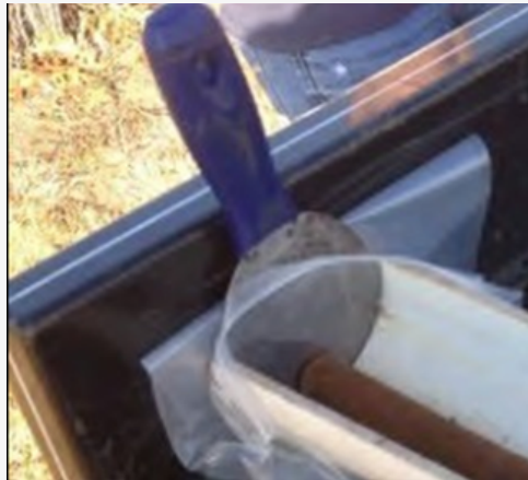
Figure 2: The spatula held firmly against the cradle assures that the core can be pushed flush to the end of the cradle before cutting. If working on the ground instead of a truck, place the hammer head and clipboard behind the spatula.
