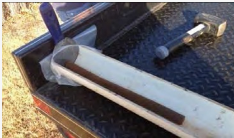
Figure 4: Core must be pushed flush to the end of the PVC cradle. This can be achieved by bracing the spatula or clipboard at the end of the cradle and pushing the dowel forward while pulling the probe back. If necessary, push the core gently forward with the spatula.
