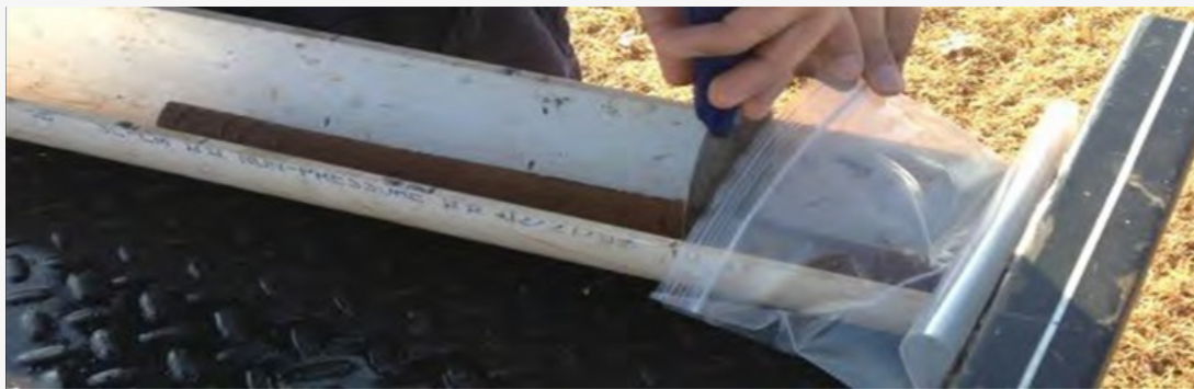
Figure 6: Core is cut at marks on the PVC cradle at 4, 8, and 12 inches from the end and pushed into labeled ziplock bags.
