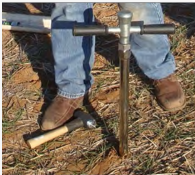
Figure 1: Probe hammered 14 inches into the ground
