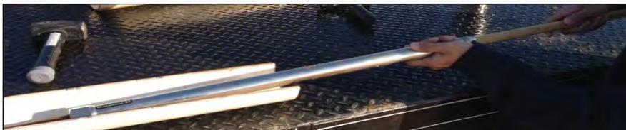
**Figure 3:** A broom stick handle with one end cut flat can be used to push the core from the probe tube.
