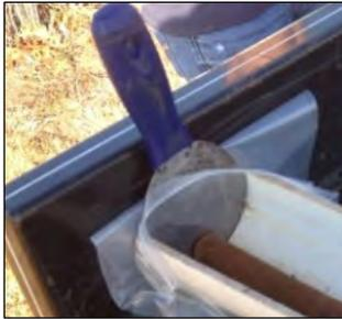
**Figure 2:** The spatula held firmly against the cradle assures that the core can be pushed flush to the end of the cradle before cutting. If working on the ground instead of a truck, place the hammer head and clipboard behind the spatula.
