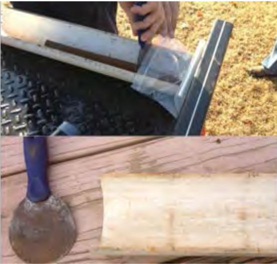
Figure 5: Rounded putty knife fits into the PVC cradle for cutting the core
