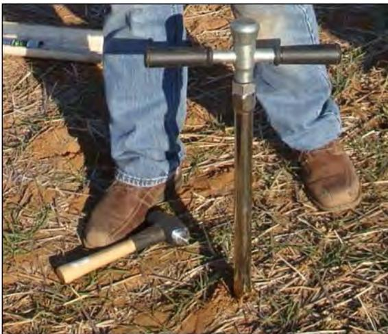
**Figure 1: Probe hammered 14 inches into the ground**
